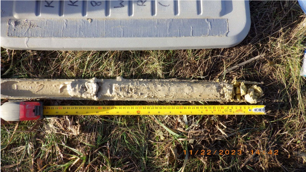
TH23-21 Photo 7: SPT at 7.2m (24 ft)
