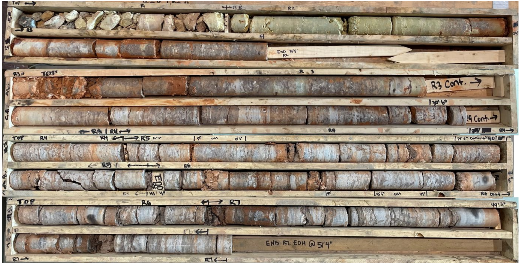
TH23-26 Photo 1: Bedrock core from 5.5 m to 15.4 m (18 ft – 4 in to 51 ft – 4 in)
