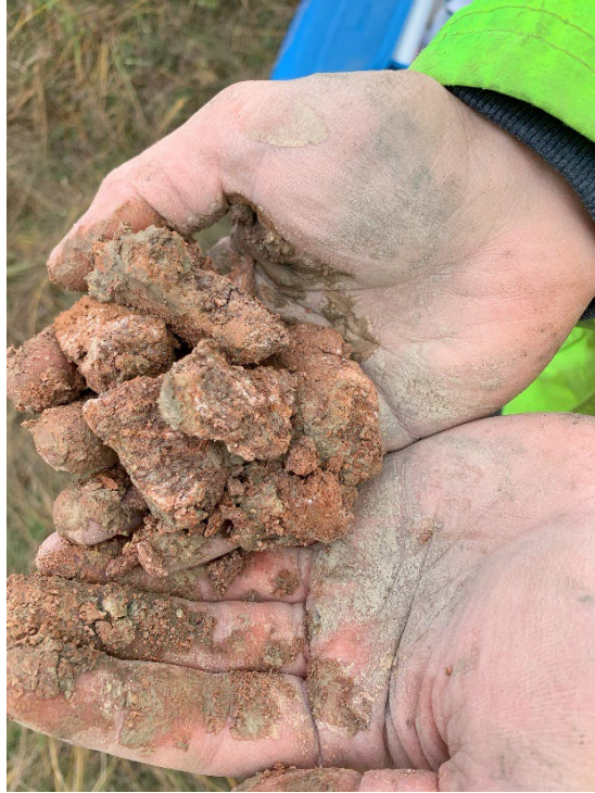
TH23-20 Photo 7: Bedrock recovered from SPT at 8.1m (27ft)
