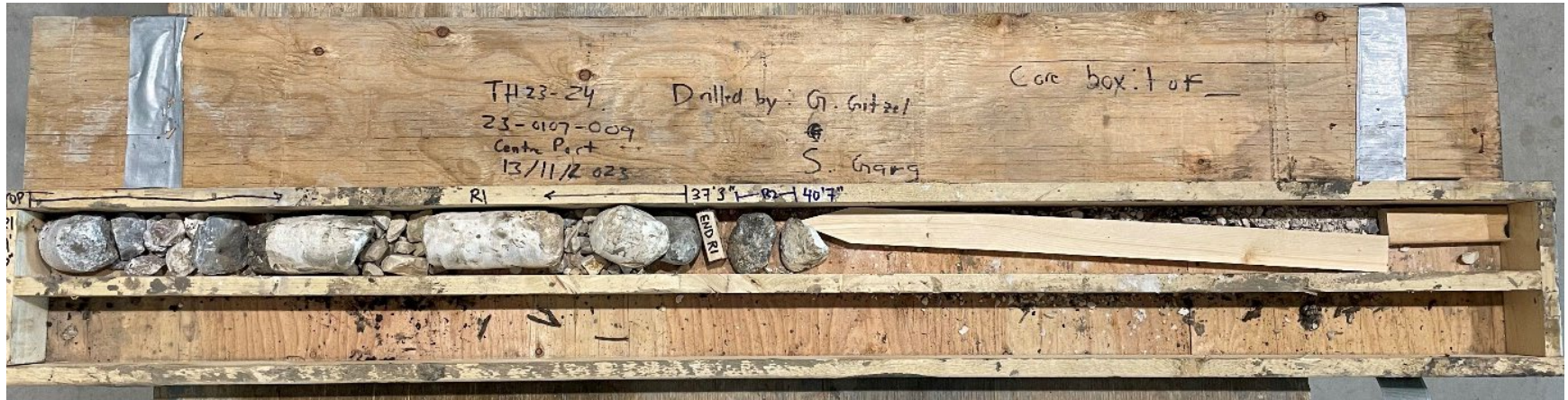
TH23-24 Photo 11: Bedrock core from 9.0 m to 11.2 m (30 ft to 37 ft – 3 in)
