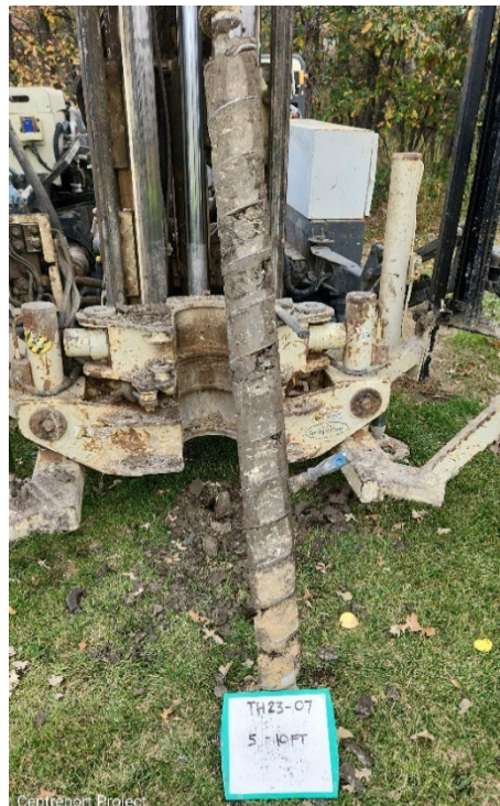
TH23-07 Photo 2: 1.5 m to 3.0 m (5 ft to 10 ft)
