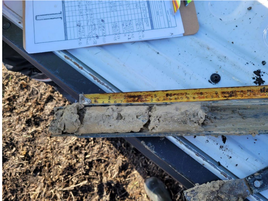
TH23-24 Photo 9: SPT at 7.5 m (25ft)
