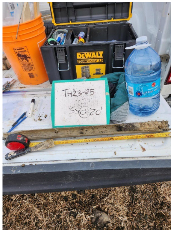
TH23-25 Photo 8: SPT at 6.0m (20 ft)
