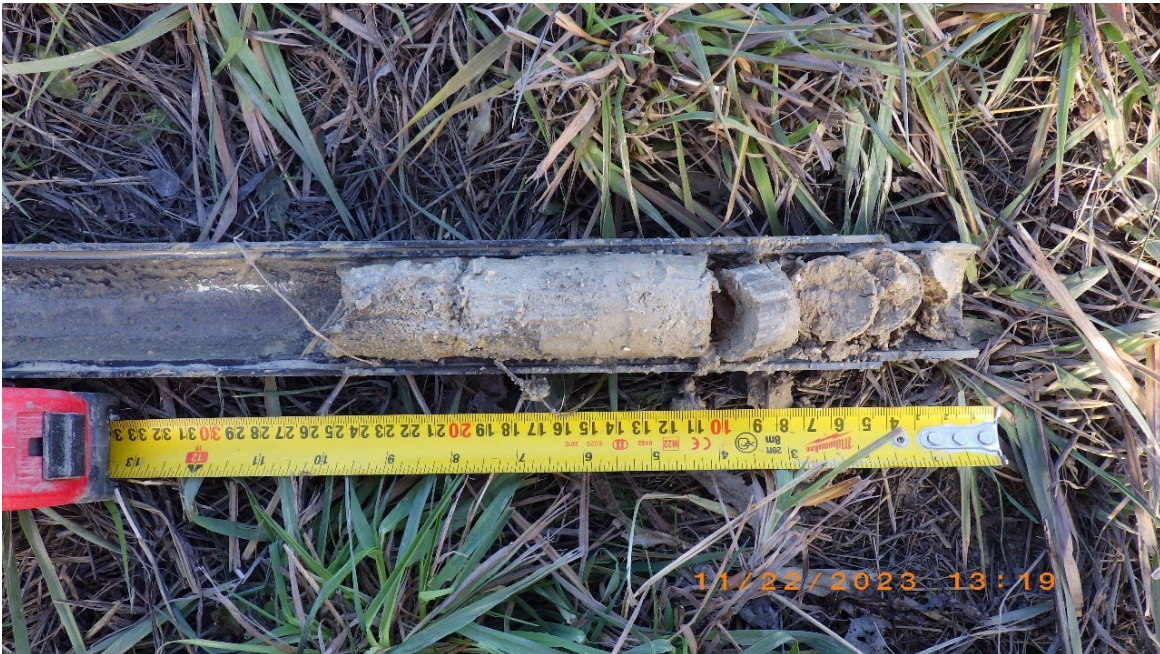
TH23-22 Photo 8: SPT at 7.2m (24 ft)
