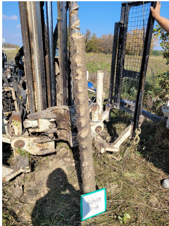
TH23-09 Photo 4: 3.0 m to 4.5 m (10 ft to 15 ft)
