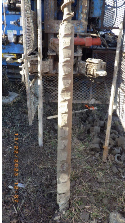
TH23-22 Photo 3: 2.7 m to 4.2 m (9 ft to 14 ft)
