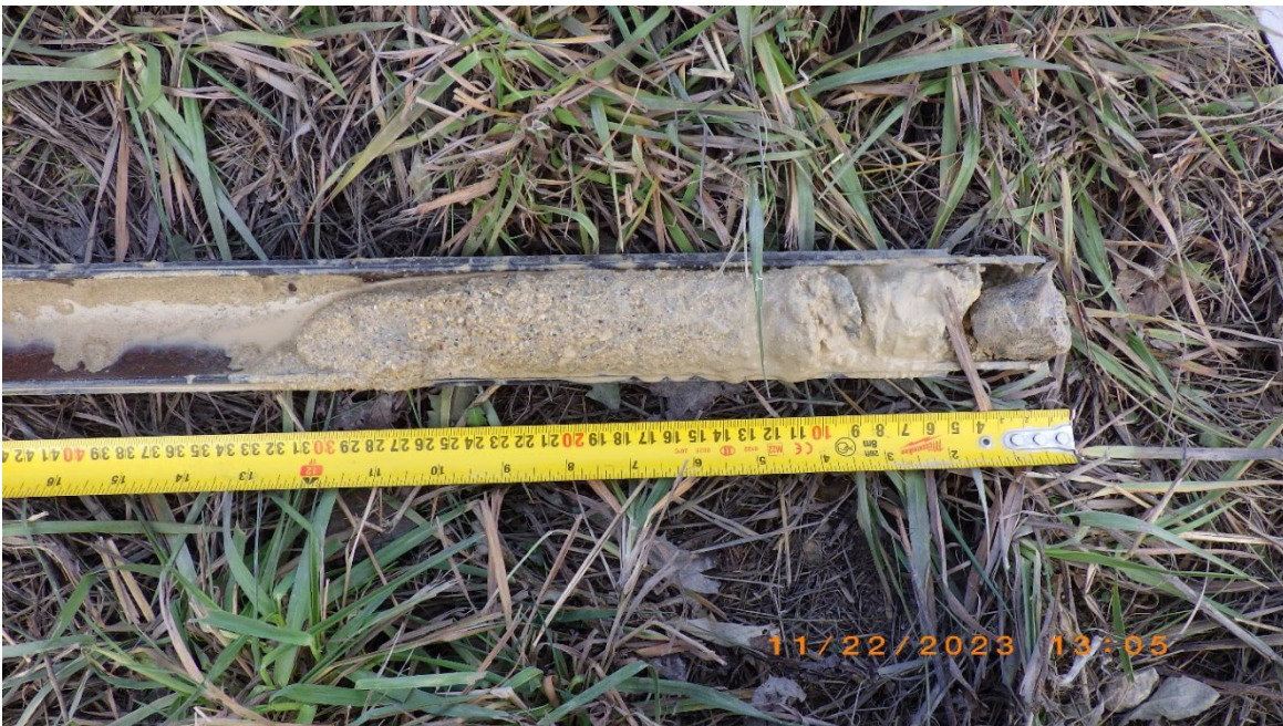
TH23-22 Photo 6: SPT at 5.7m (19 ft)
