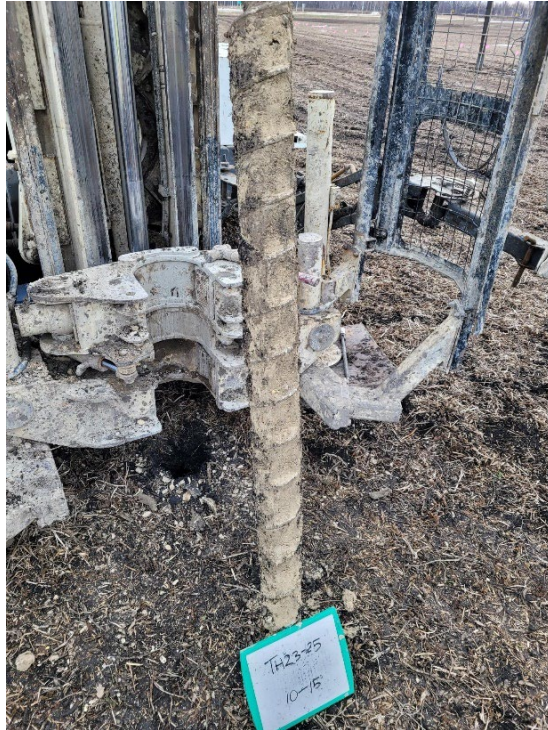
TH23-25 Photo 3: 3.0 m to 4.5 m (10 ft to 15 ft)
