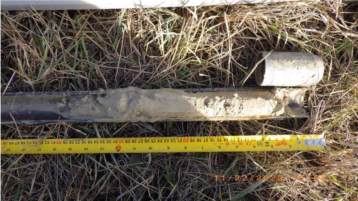
TH23-23 Photo 5: SPT at 5.7m (19 ft)
