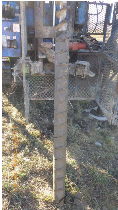
TH23-21 Photo 2: 1.2 m to 2.7 m (4 ft to 9 ft)
