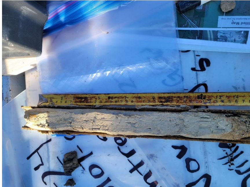
TH23-24 Photo 7: SPT at 4.5 m (15ft)
