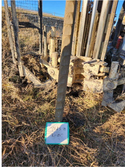
TH23-19 Photo 3: 3.0 m to 4.5 m (10 ft to 15 ft)
