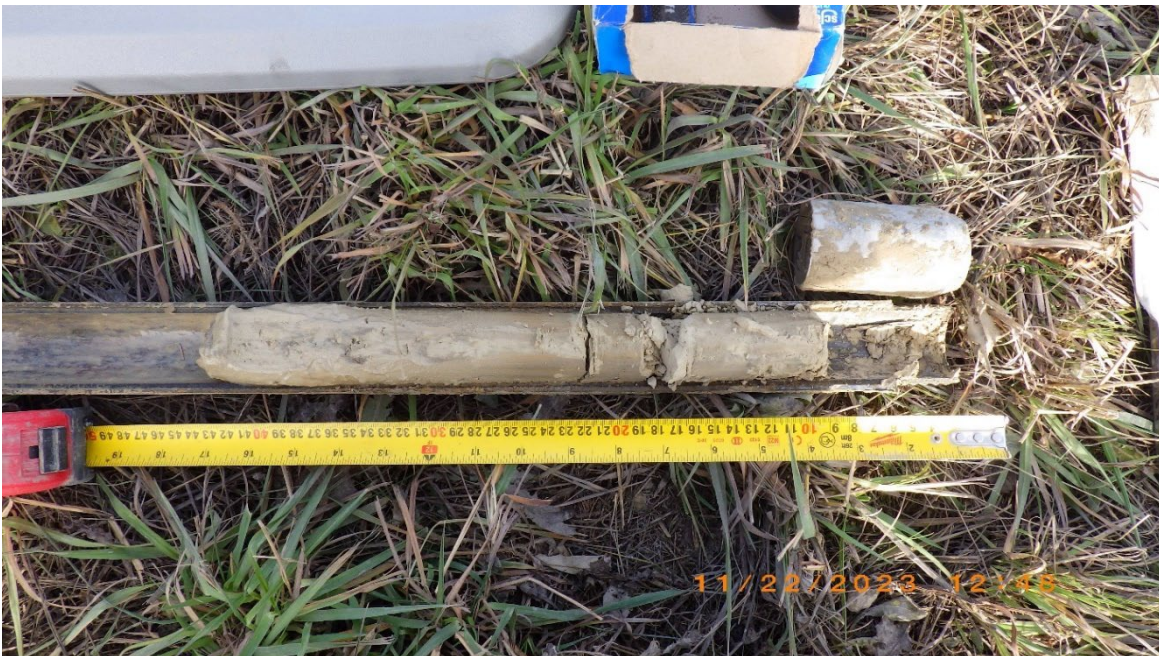
TH23-22 Photo 4: SPT at 4.2m (14 ft)
