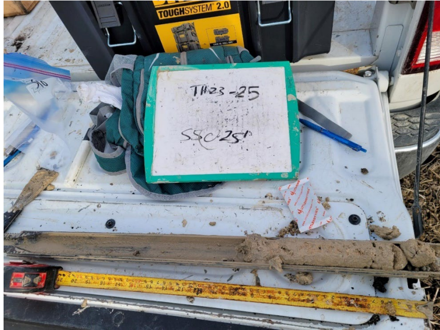
TH23-25 Photo 9: SPT at 7.5m (25 ft)
