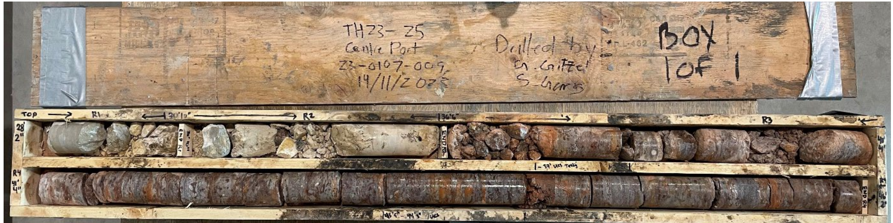
TH23-25 Photo 10: Bedrock core from 8.5 m to 13.9 m (28 ft – 2 in to 46 ft – 2 in)
